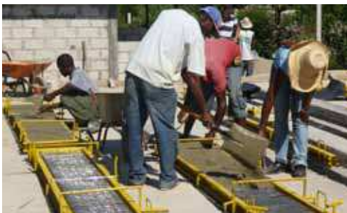
A mobile vibrator forms the panels (above). Alternatively panels are produced by hand (below). © Ecosur.
